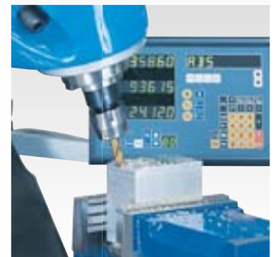
cutter head swivels \pm 360^\circ
