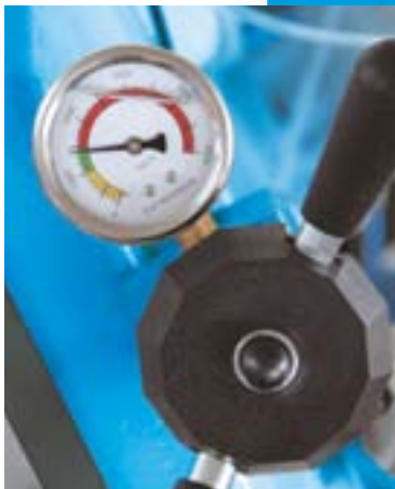
pressure gauge for saw blade tensioning
