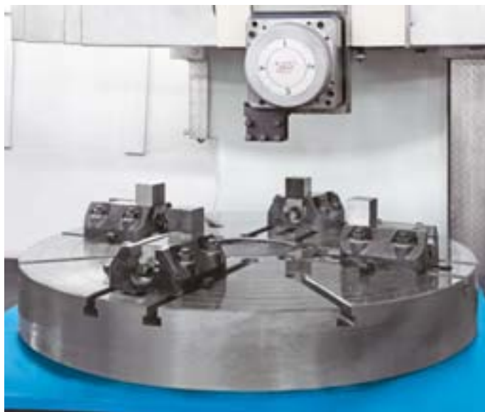
face plate with 4-station tool changer
