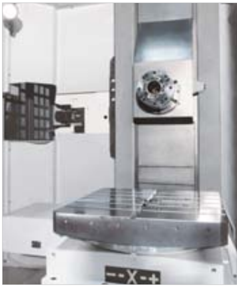
rigid moving column design
