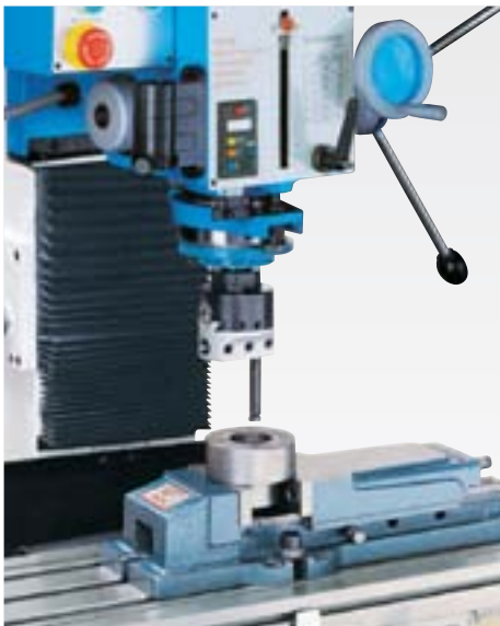
inside diameter boring and facing
