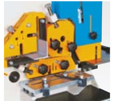
angle steel station
