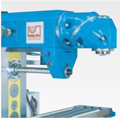
Horizontal milling with rigid outer arbor support
