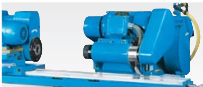
swiveling headstock with cylindrical grinder
