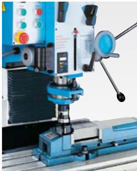
milling with milling arbor
