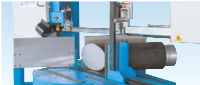
exact angle adjustment with digital display
