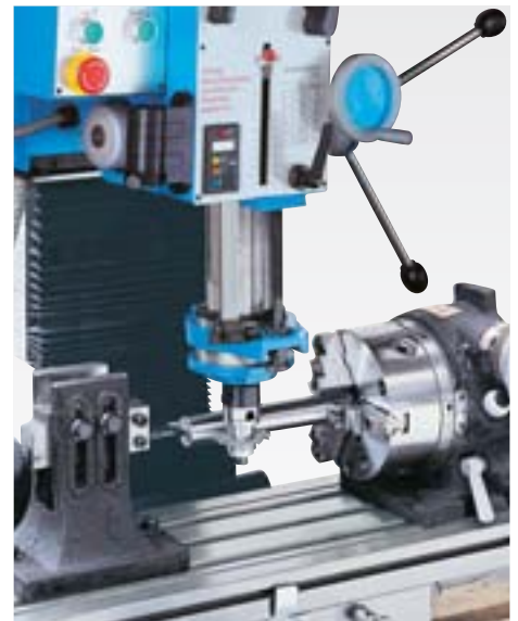
slot cutting with divider
