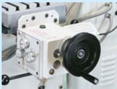
feed gears with rapid feed
