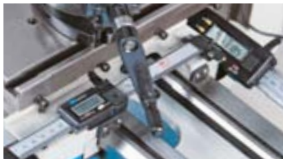
Digital length measuring system on Z and X axes
