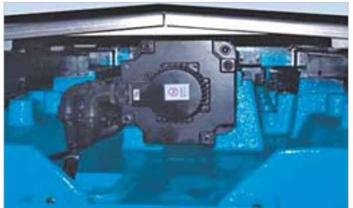
servo drives on all 3 axes
