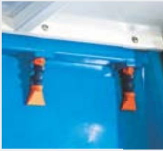
Chip Flushing System
