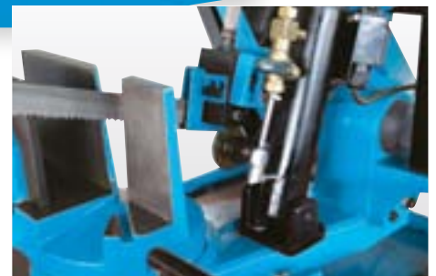
pressure gauge for saw blade tensioning
