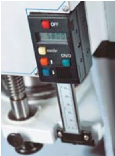
digital drilling depth indicator
