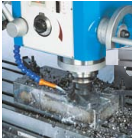
face milling with cutter head
