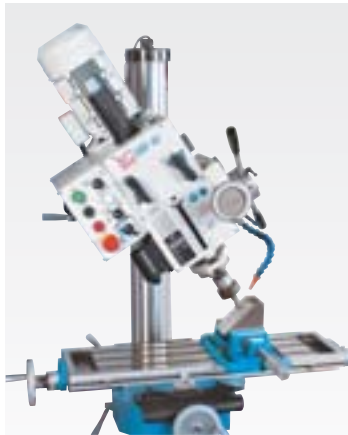
cutter head swivels to both sides
