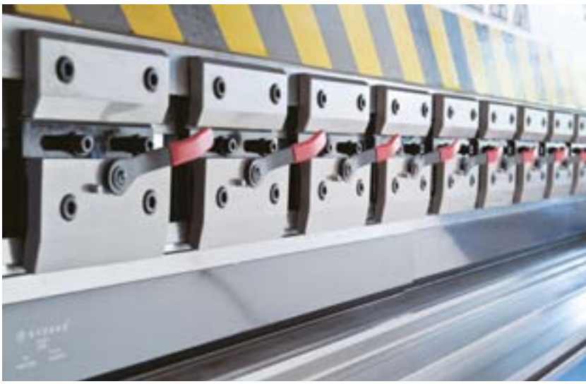
quick-change system for male die
